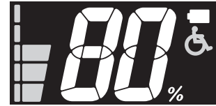
Battery residual capacity indication
